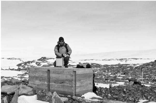
Figure 2: Gravimetric local tie measurements at Novolazarevskaya during FINNARP 2011.
